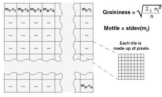
Figure 1. Image area is divided into a number of tiles for calculating graininess and mottle.
