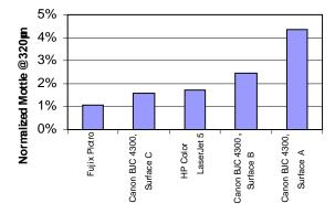
Figure 7. Normalized magenta mottle measurements.
