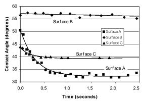
Figure 9. Stabilization of contact angle with time.
